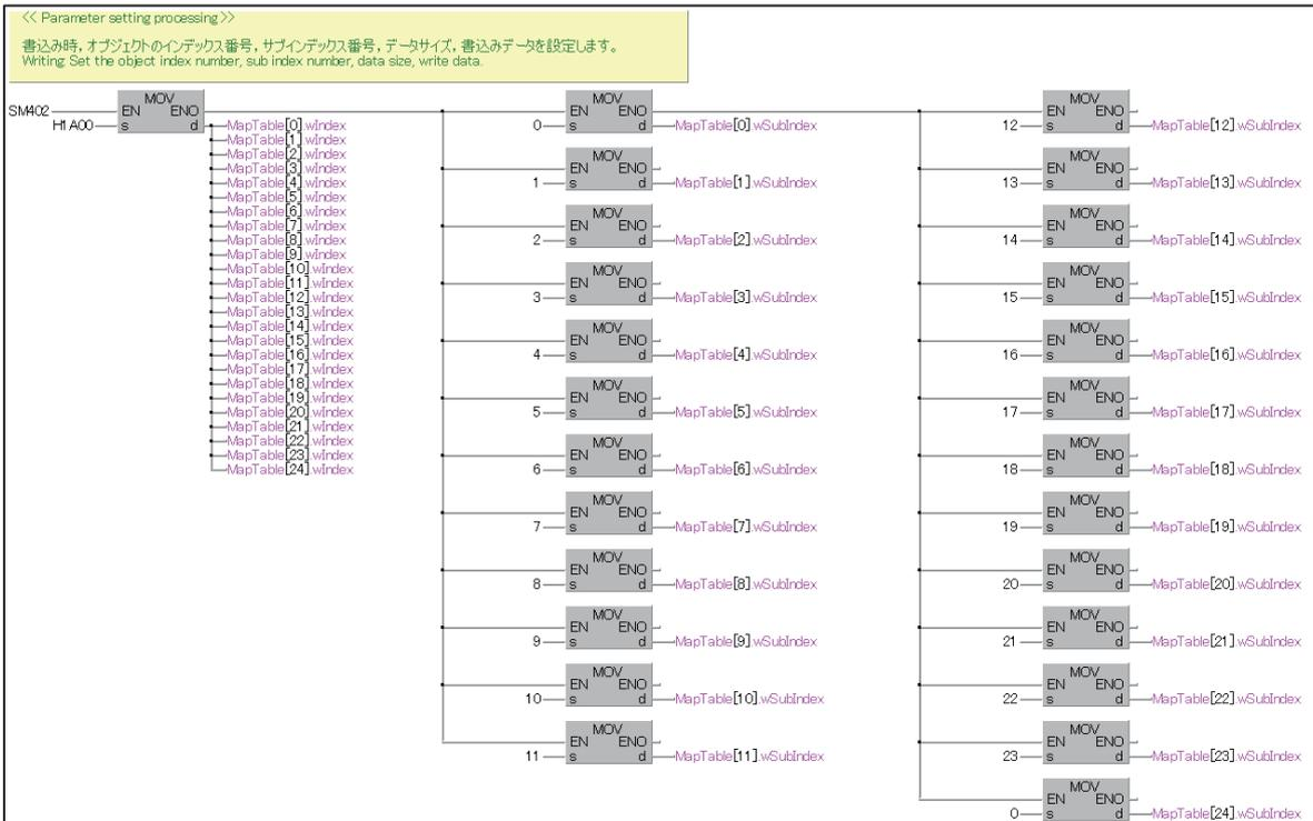
The start [0] and end [24] of the table set the number of components, and [1] to [23] set the mapping data.
